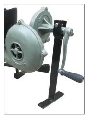
PART-A is to be fitted on the hole provided on the Iron Furnace with the help of 12x13mm Ring Spanner.
