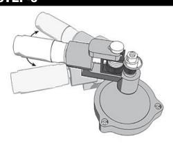
Continue tightening while rotating the handle 360 degrees to stretch a plain band or back and forth for a ring with stone setting.
