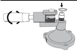
• Place the ring to be stretched on the shaft which is attached to the base and tighten the handle.
