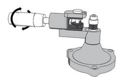
Turn the chrome plated handle counter clockwise to open die – pin attachment.
