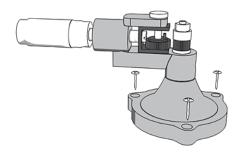
• Attach the ring stretcher to a sturdy surface (screws not included).
