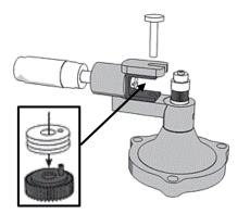
• Lift the knurled pin, place the selected die on top of the black gear (the hole in the die goes over the peg on the gear), then replace the pin.
