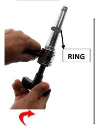
Insert the ring into conical spline, now ring is ready to be stretched. Hold the grabbing handle with one hand and rotate the rotary handle clockwise with the other hand for 4 to 5 rotations. Flip the ring and repeat this process until the size of the ring increases by one increment.
