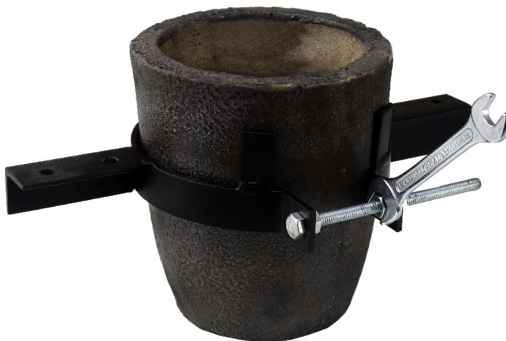
(STEP-3) Check your crucible in the Pouring tongs ring. After final assembly, tighten all bolts with a spanner.
