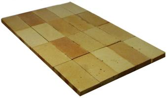
Place Forge over the plain surface. You may prepare it by placing refractory bricks or by using castable cement which can withstand high temperatures.
